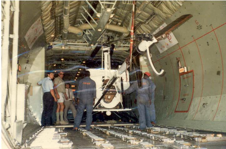
**Hughes 300C helicopter being loaded into the Lockheed Hercules C-130 aircraft.**
